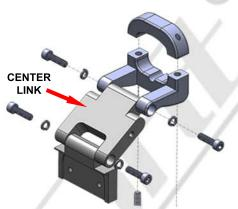
5 - The center-link may be removed if an overall shorter mount length is needed, depending on your rear view miror and desired position for the RD. With multiple adjustments available, you should be able to postion your RD right where you want it. If you are unable to achieve this, be sure to contact us at 1-707-664-8234
